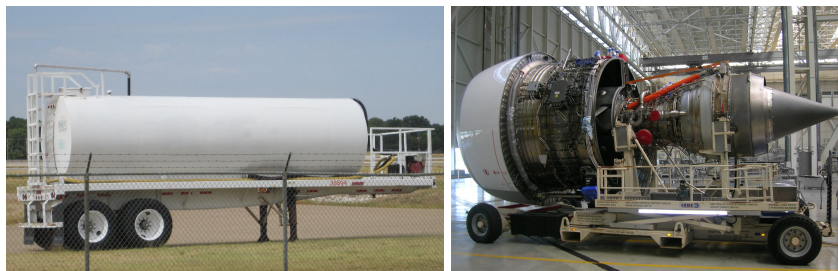
Figure 1.2: A trailer, with zero power ( \dot{Q} = 0 \text{ W} ) but capable of delivering a lot of energy. The combustion of 20 t of kerosene releases about Q = 800 \text{ GJ} as heat; A Trent 900 turbofan engine, with very high power (able to supply \dot{W} = 14 \text{ MW} to a commercial aircraft) but devoid of energy (0 J).
