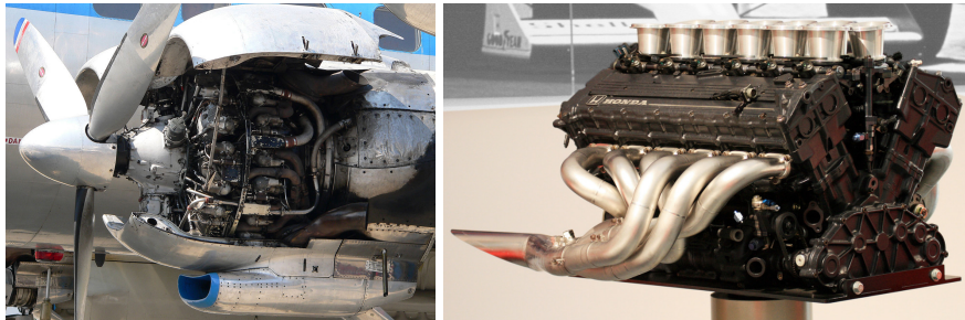
Figure 10.6: On the left, a 1950 Curtiss-Wright R-3350 Duplex-Cyclone of 3500 hp with 18 cylinders arranged in two successive rows. Four of these engines powered the long-range aircraft Lockheed Super Constellation . On the right, a 1991 Honda RA121E V12 engine. It powered the McLaren MP4/6 Formula 1 car.
