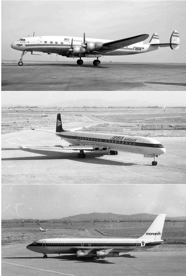
Figure 9.26: From top to bottom: The 1943 Lockheed Constellation , the culmination of the propeller aircraft era: four Wright Duplex-Cyclone supercharged 18-cylinder engines, capable of covering 3700 km (2300 mi) at 500 km/h (310 mph). The 1949 De Havilland Comet , the first jet airliner: four Halford Ghost turbojet engines, capable of covering 2400 km (1500 mi) at 740 km/h (460 mph). The 1957 Boeing 707 , with a configuration and performances anticipating those of all its successors: four Pratt & Whitney JT3C turbojet engines, capable of covering 4300 km (2700 mi) at 900 km/h (560 mph).
