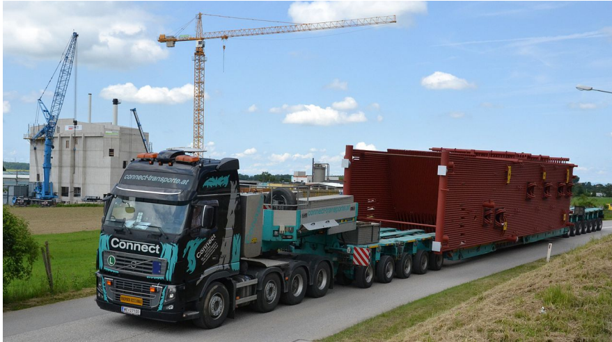
Figure 9.3: Transport of the boiler for a wood power plant capable of withstanding a pressure of 100 bar.
