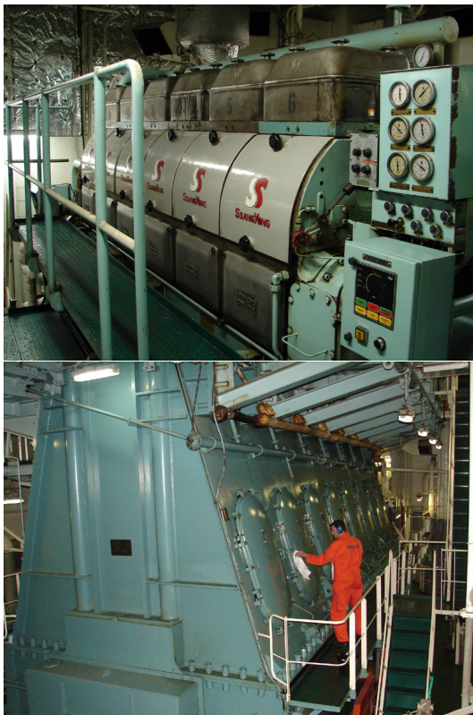
Figure 10.32: The two Diesel engines of a 290.000 t oil tanker: a six-cylinder 1100 kW generator (top) and a seven-cylinder 25 MW propulsion engine (bottom).
