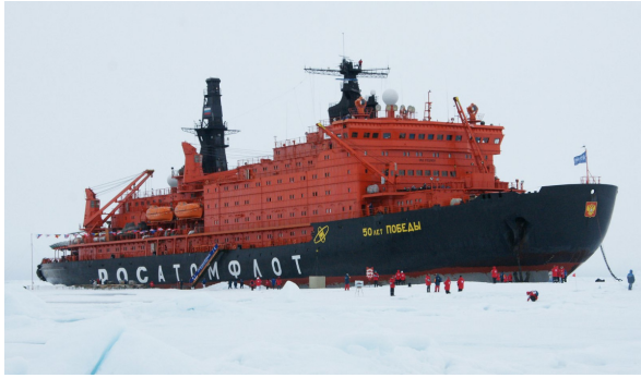
Figure 9.28: The 50 Let Pobedy , a 25,000-ton nuclear-turbo-electric powered icebreaker (two reactors of 171 \text{ MW}_{\text{heat}} , three engines of 17.6 \text{ MW}_{\text{mech.}} ). Its construction started in 1989 but it only entered service in 2007.
