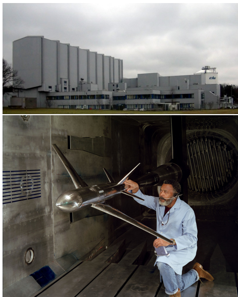
Figure 6.20: Buildings of the ETW (European Transonic Windtunnel) in Cologne and test section of the National Transonic Facility of NASA, of similar size and capabilities.
