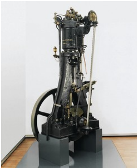
Figure 7.14: The second prototype developed at MAN by Rudolf Diesel, and the first to operate independently, in February 1894. It has only one cylinder with a diameter of 22 cm, and the direct fuel injection is done by a compressed air circuit. The engine is now exhibited at the headquarters of the MAN company.
