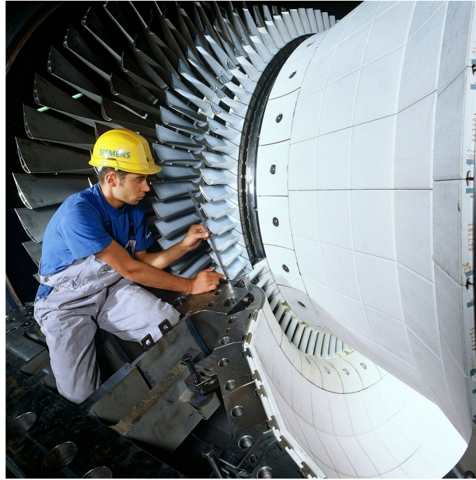
Figure 10.12: Turbine of a gas generator. The photographed turbine, a Siemens SGT5, can accept an air and water flow rate of 690 \text{ kg s}^{-1} (1521 lb/s). It delivers approximately 500 MW of shaft power.
