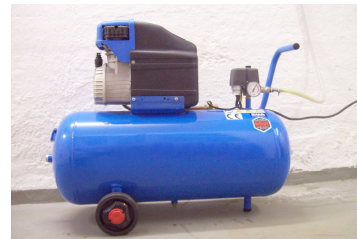
Figure 4.15: A small electric compressor mounted on a portable air tank
