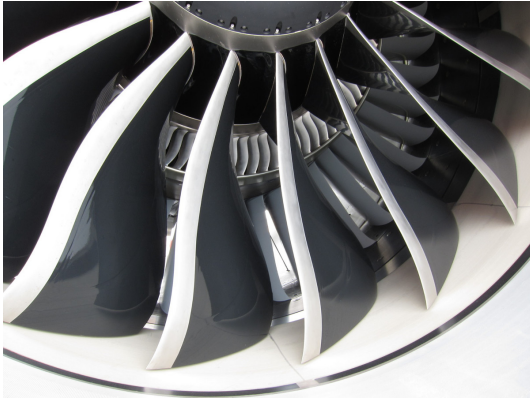
Figure 4.17: Air intake of one of the four General Electric GENx-2B turbofans equipping a Boeing 747-8. The two-color fan blades are visible in the foreground; behind, the air flow is divided between the compressor inlet (internal) and the cold flow rectifier stators (external).
