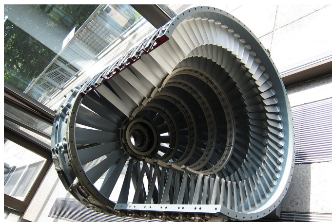
Figure 10.8: The stator casing which houses the rotor (not shown) in the an axial compressor of a turbojet engine.
