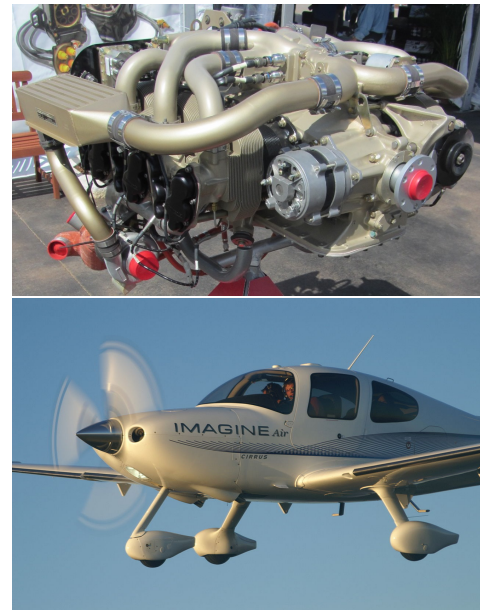
Figure 10.31: The 300 hp six-cylinder gasoline fuel injection Continental IO-550, in production since 1983. It equips among others the Cirrus SR22 aircraft. This photo shows the turbocharged version of the engine, with the intercooler visible in the top left corner.
