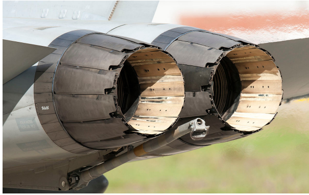
Figure 10.14: The nozzles of two General Electric F404 engines equipping a fighter aircraft. The geometry of the nozzle (not covered in this book) is programmed to adapt to the engine mass flow and whether or not afterburning is used.
