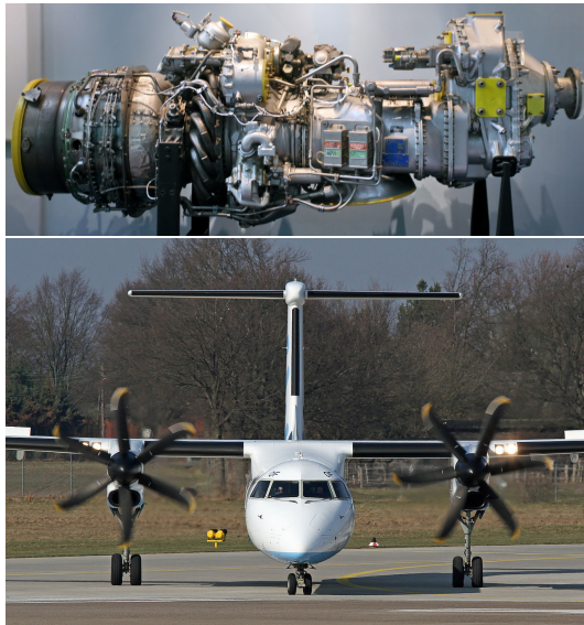
Figure 10.34: A Pratt & Whitney Canada PWC123 turbo-prop engine powering a Bombardier Dash 8. The PWC123 is configured with three concentric rotating assemblies, with the engine shaft powered by a free turbine, but its operation principle remains similar to that described in figure 10.33.
