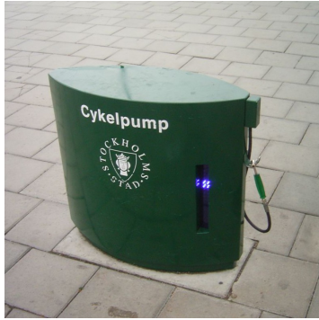
Figure 8.15: Public air compressor in Stockholm for cyclists. A heat exchanger integrated under the bodywork fortunately ensures the temperatures calculated in this problem are never attained.
