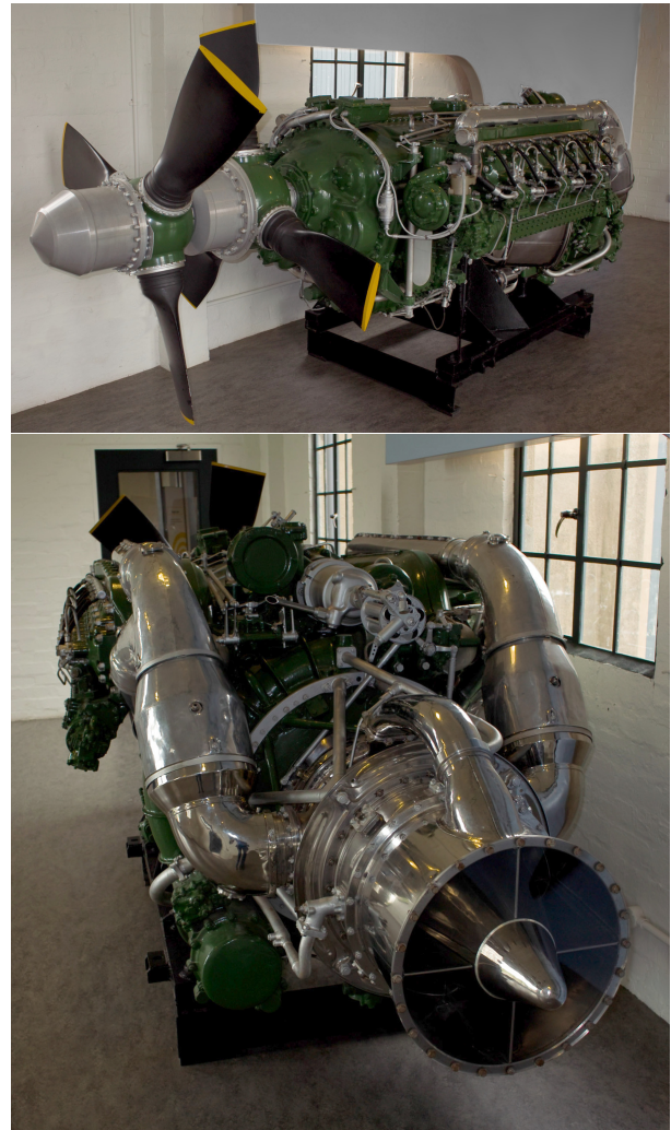
Figure 10.28: The prototype of the Napier Nomad I . The displacement was 40 L and the weight exceeded 2 tons.
