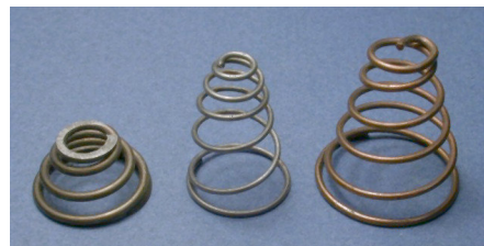
Figure 1.9: Conical springs, whose stiffness increases exponentially when compressed. We will see in chapter 2 ( closed systems ) that when fluids are compressed and expanded slowly, they behave similarly to spring C, which has a conical geometry like those shown here.
