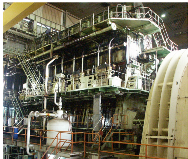
Figure 7.16: A nine-cylinder Sulzer RTA76 Diesel engine producing 25 MW of power at 95 rpm. This unit is installed here in a factory but the model is commonly used to propel merchant ships.
