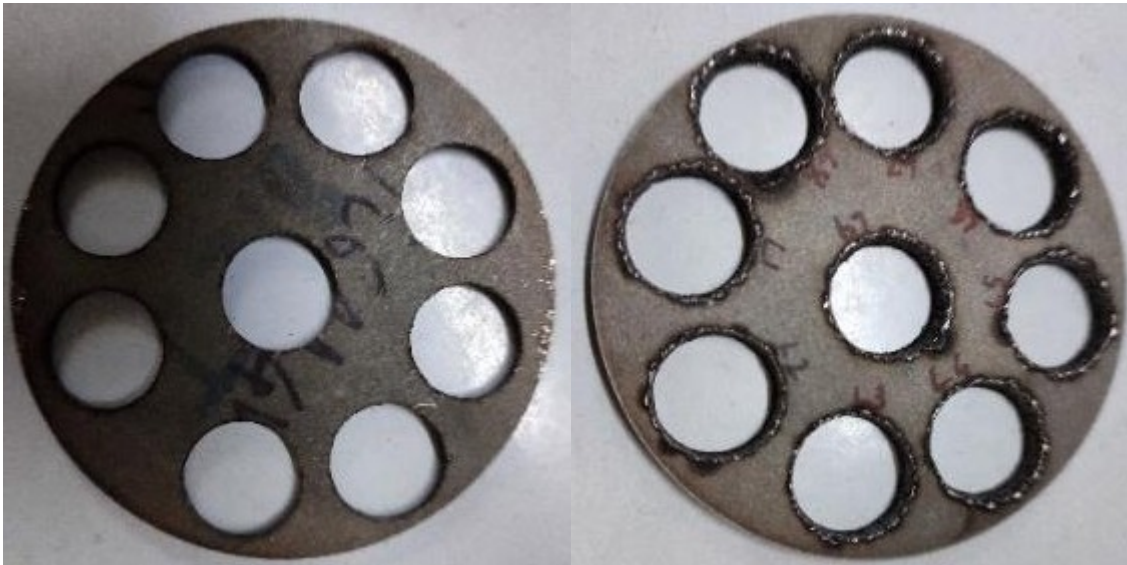
Fig. 5(a) Ti64 – GA mist (b) Ti64 – EDM oil
