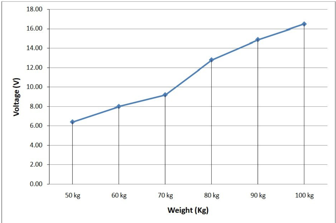
Fig.2-Output Voltage Depends on Weight (Kg) at 1*1 Feet tile
