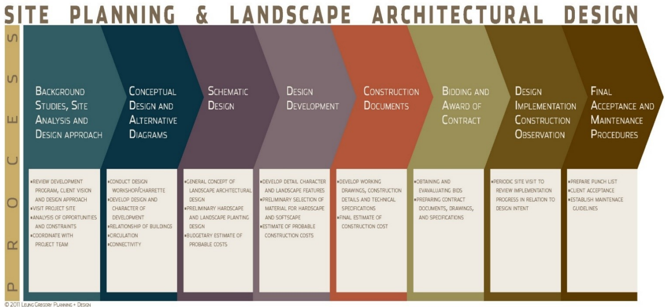
Figure: Typical design-development progression toward construction documentation.
