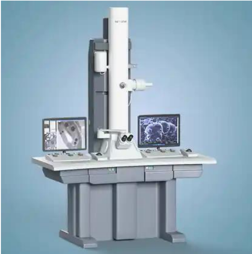
Figure 5. Transmission electron microscope used for nanoscale characterization
