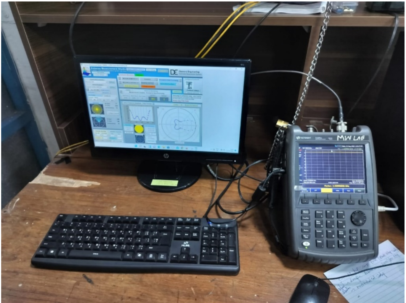
Figure 16 (b) Reading setup for Anechoic chamber
